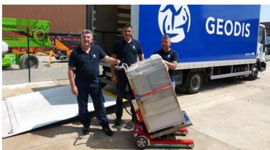
Electric hand truck to carry the heavy and bulky loads in staircases
